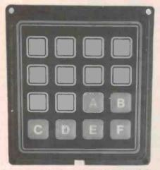
You can substitute a standard hex keypad, like this one, for the Jerry-built one I used. You'll still need pull-up resistors. Eight pins on the back will be marked '1' to '8'. Pins 1 to 4 connect to pins 1 to 4 of Port A. Pins 5 to 8 on the keypad connect to pins 1 to 4 of Port B.
