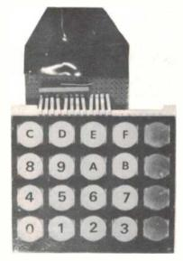
I made this hex keypad from an old calculator board — it's cheap, simple and effective!
