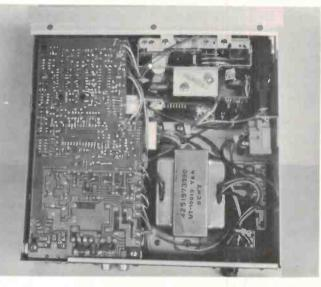
The channel separation is only modest, achieving less than 48 dB separation at mid-band frequencies and 30 dB separation in the 6 to 12 kHz region. The signal to noise performance is, however, substantially better than I would have expected in such a small unit, being 59.5 dB(A) relative to the +6 dB signal and 53.5 dB(A) relative to the zero dB level.
